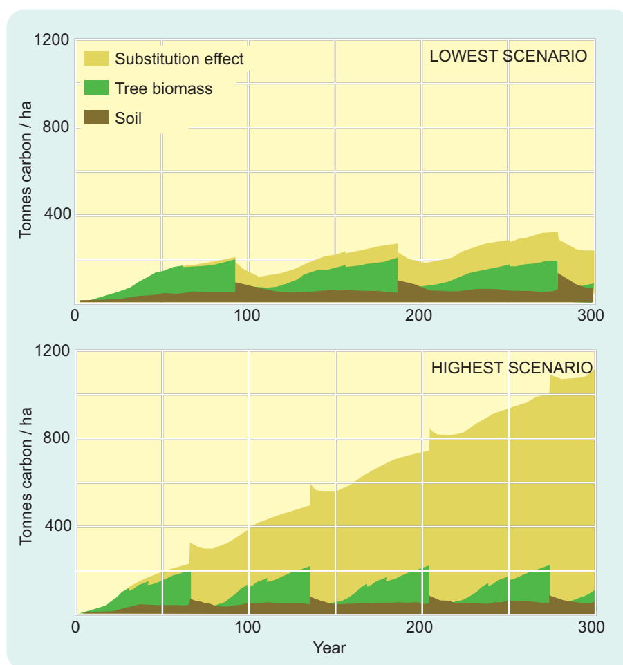
Figure 12. Stored carbon in tree biomass and soil, and the cumulative effects of materials substitution for two scenarios. The upper graph, with the least positive climate effect, is based on present-day forestry, with no harvesting of stumps or logging residue, and takes natural gas as the reference fuel. The lower graph, with the highest positive impact on climate, is based on intensive forestry with stump harvesting, extensive materials substitution, and takes coal as the reference fuel. (After Eriksson et al. 2007.)
