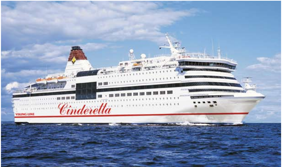
By fitting SCR to all its engines, the emissions of NO x from Viking Line's MS Cinderella are cut by 97 per cent, down to 0.5 g/kWh. It also uses low-sulphur (<0.5%) fuel, and is in Stockholm connected to shore-side power. In early 2013, Viking Line will introduce a new ship serving the Turku-Åland-Stockholm line and operating on liquefied natural gas (LNG).
